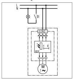
The F fan is designed for installation in windowless, dark rooms. The unit is switched on wirelessly through the brightness of the room lighting by a light control unit. The unit starts up after approximately 50 seconds.
